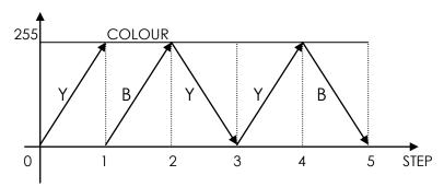
All lights operate synchronously with a fade effect.
