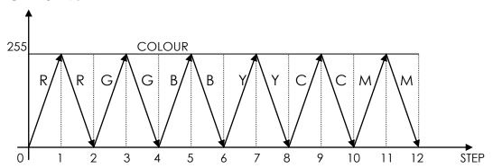
All lights operate synchronously with a 7 color fade effect.
