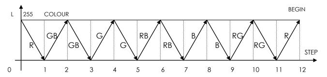
All lights operate synchronously with a fade effect.
