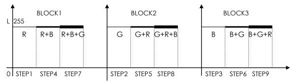
Divide the 12 steps into 4 parts (BLOCK1, BLOCK2, BLOCK3); there is no fade effect.
