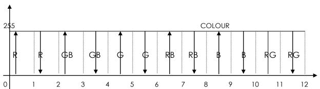
explanation all BLOCK are synchronization without fade effect and keep the COLOUR in highest brightness.
