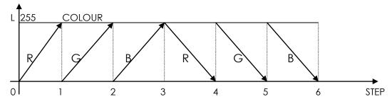
All lights operate synchronously with a fade effect.
