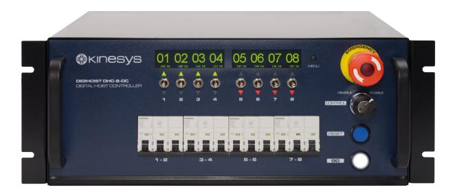
At the core of the system is a digital communications link that enables multiple units to be daisy chained together. The units will **automatically assign channels** according to their position in the daisy chain. The high resolution displays offer comprehensive channel feedback including channel number, status and load cell information.
