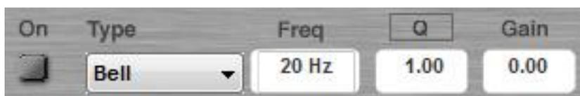
Both input channels have up to ten parametric EQ's. Each parametric equalizer can be configured as an Allpass, Bell, High shelving, Low shelving or a Notch filter.
