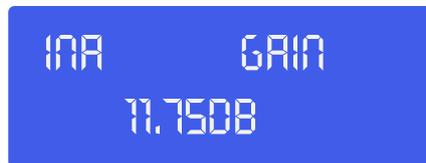
Adjust the gain by dialing the **jogwheel (8)**. Push the **item up (2)** button to proceed with the next item. In our example the Lowpass filter.
