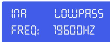
Adjust by dialing the **jogwheel (8)**. You can switch the lowpass filter off by dialing the **jogwheel (8)** clockwise until the frequency passes 20kHz. Click the **jogwheel (8)** to change the filter type.
