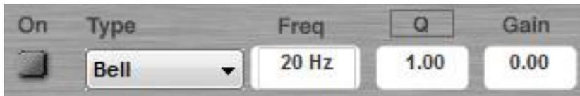
Both input channels have up to 5 parametric EQ's. Each parametric equalizer can be configured as an Allpass, Bell, High shelving, Low shelving or a Notch filter.
