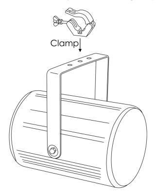
The PSB-510M can be mounted to any kind of truss with a clamp.
